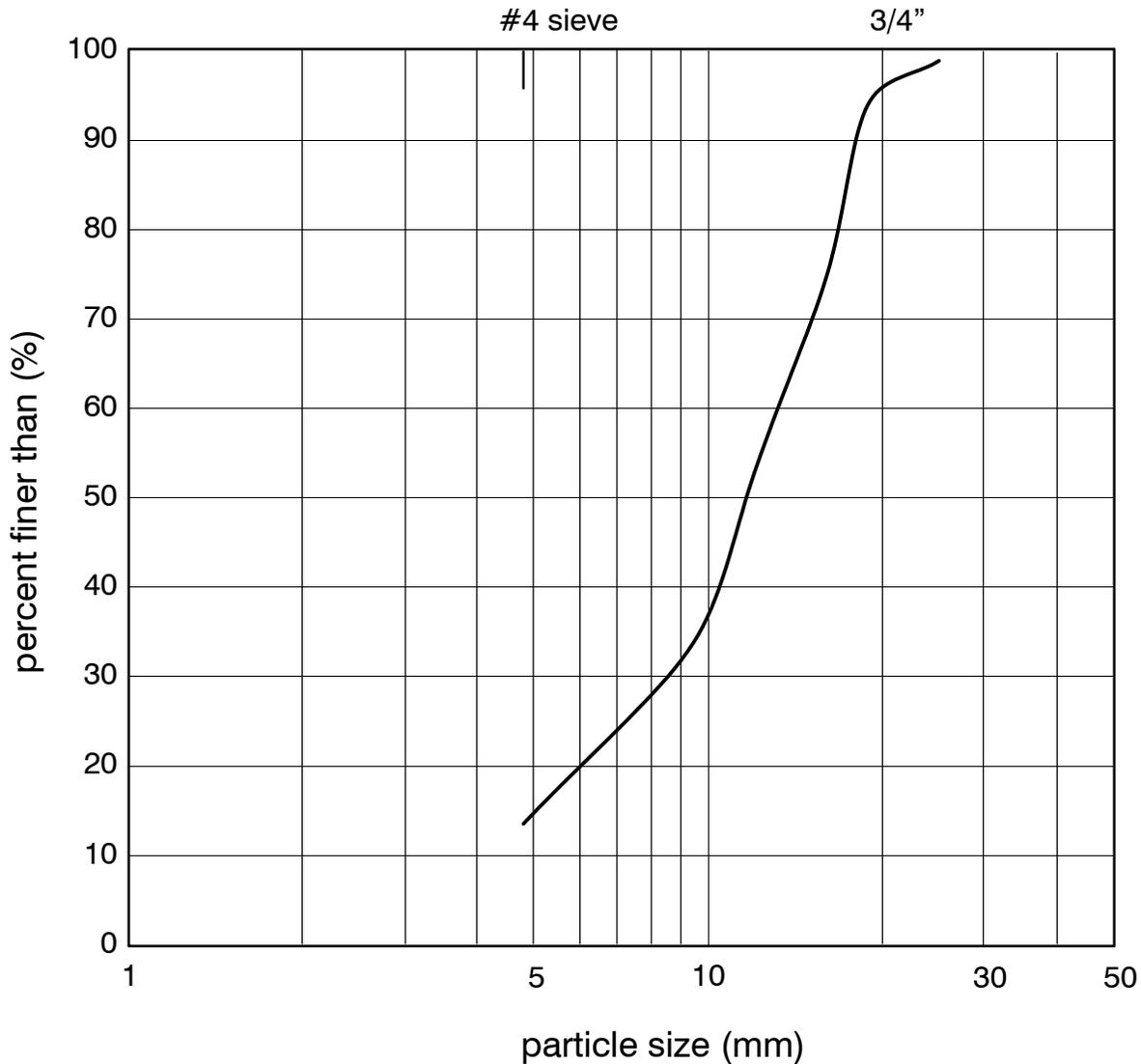
Figure 2: Particle size distribution for 100% crushed granular stone used in RR-N 115 block tests
